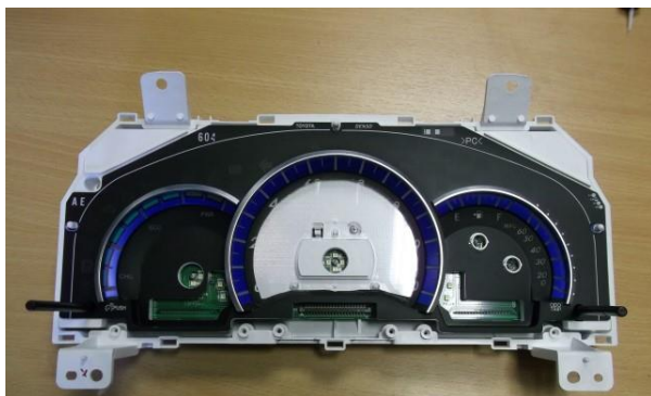
REPOSITION FASCIA ON CLUSTER BACK PLATE. POSITION NEW DIAL IN PLACE AND REFIT PLASTIC COLLARS.
