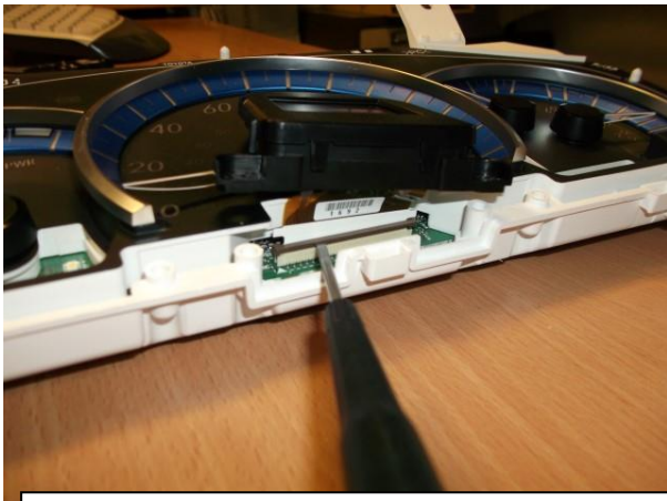
CAREFULLY DISCONNECT RIBBON CABLE
