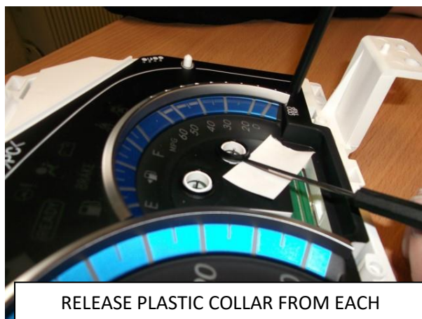
CAREFULLY REMOVE NEEDLE/POINTER
