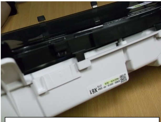
REMOVE FRONT COVER BY RELEASING CLIPS
