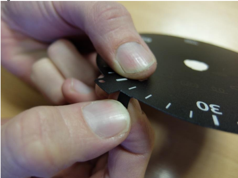
Fig 2: Locate tab down into existing hole under white clip.
