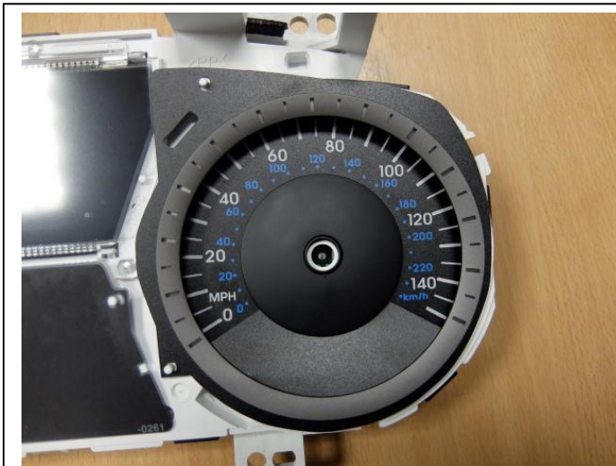
9: Clip on original outer bezel.
