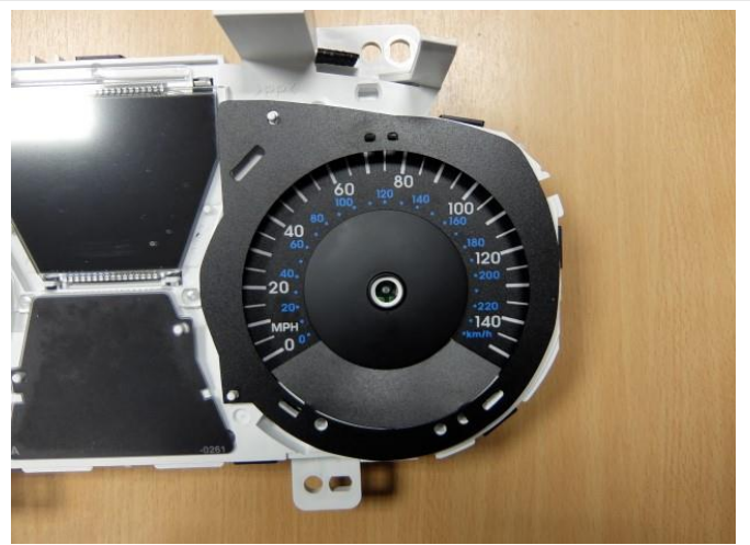
8: Position the outer ring panel.
