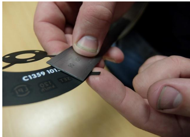
3: Crease each tab at the point shown here.
