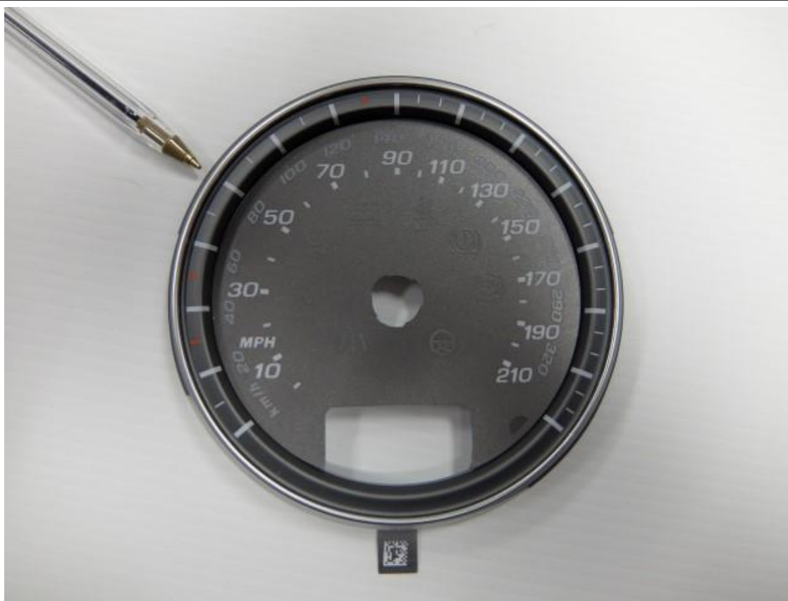
Step 3 - Seating the new dial face. Line up the 50 MPH with the 80 KMH.
