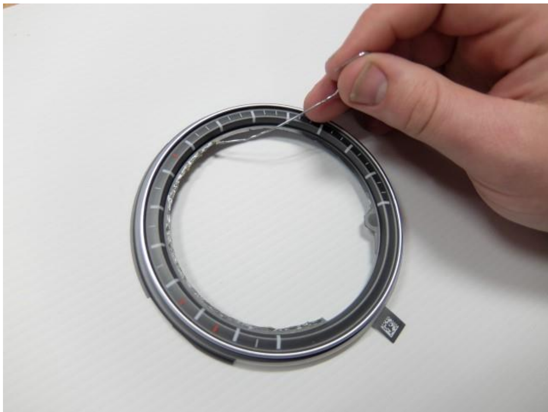
Step - 2 Carefully apply a small bead of SOLVENT FREE glue to the inner edge of the shelf / lip. Keep the glue 1mm away from the outer ring.
