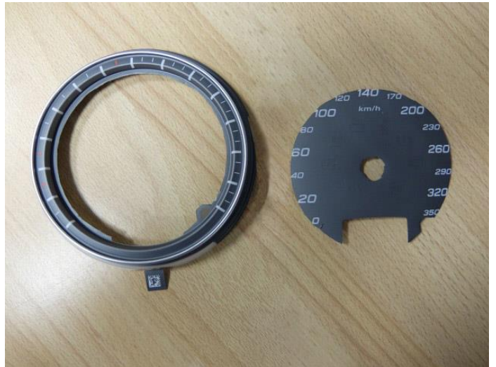
Step - 1 Cut out the center and leave a small (2mm approx.) shelf / lip.
