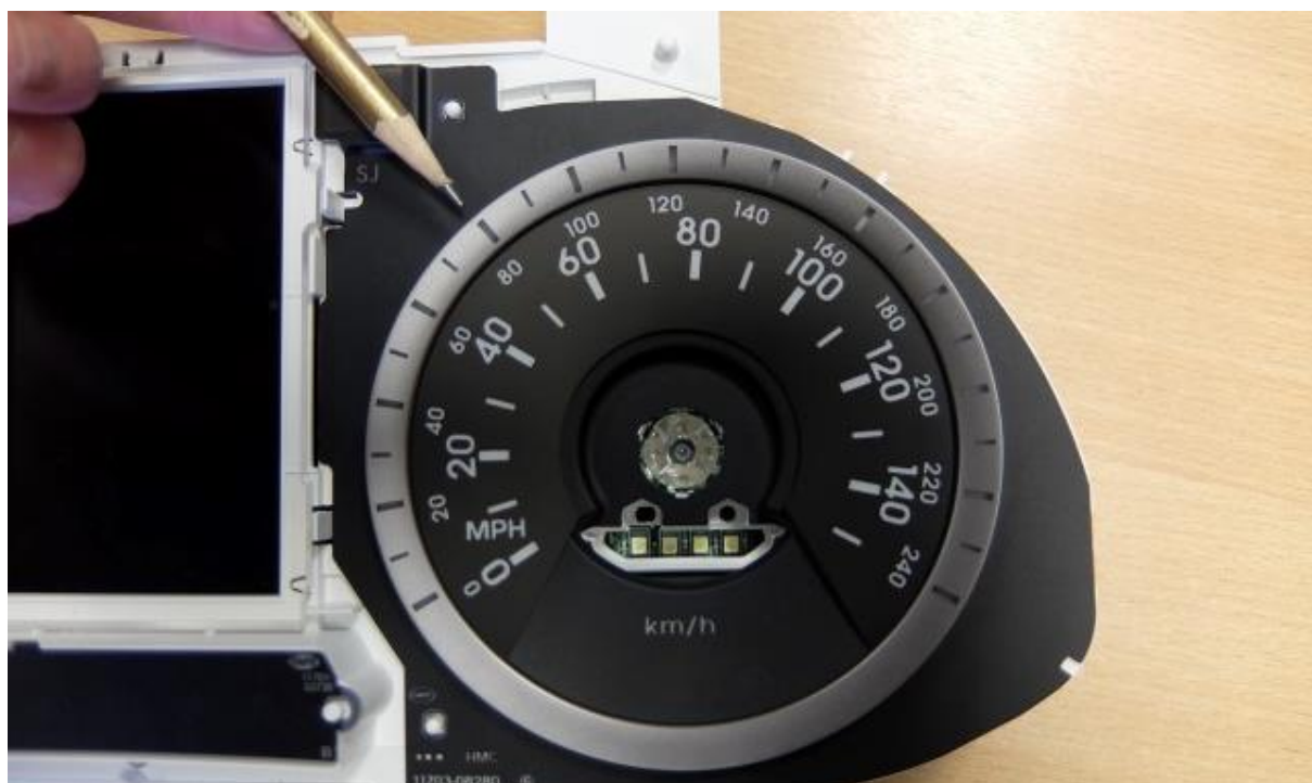
Position the replacement MPH dial under the bezel ring and line up 50 MPH with the 80 kmh marks (& 150 MPH with 240 kmh) and replace the retaining collar.
