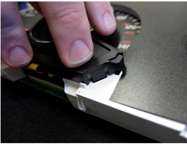
13: Refit the digital display (see Step 14 too).
