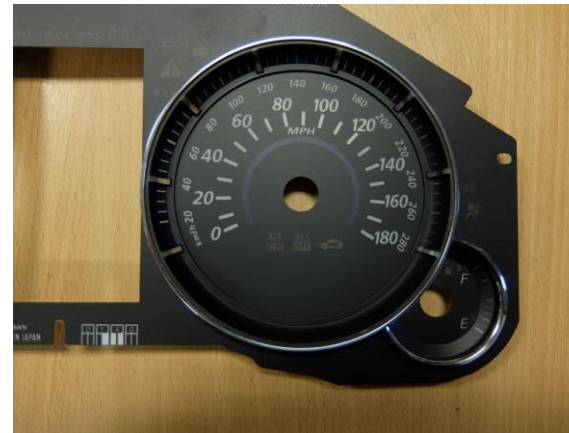
5) Refit the calibration ring
