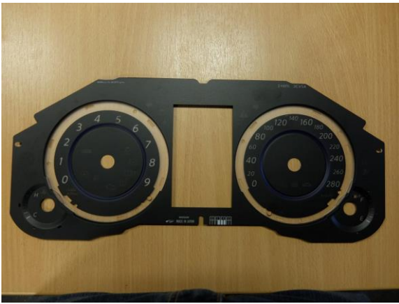
1) Original dial fascia with calibration ring removed
