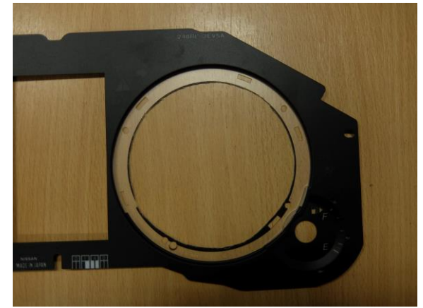
3) Centre cut out leaving ALL locating holes
