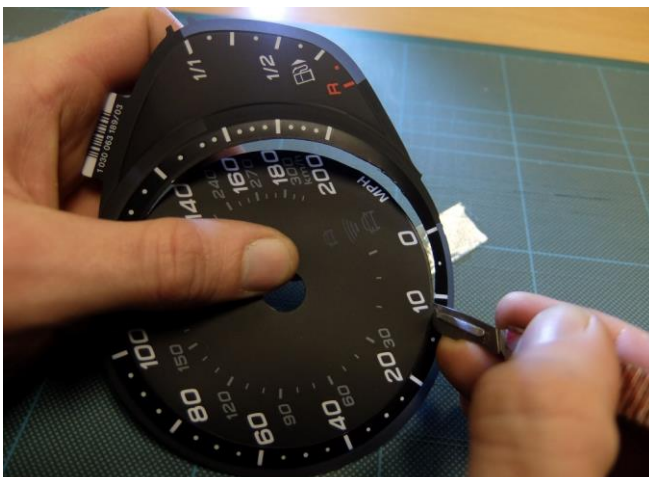
1: Using a craft knife cut out the original dial centre
