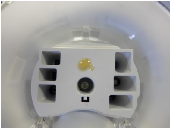
10) Apply a small amount of adhesive to the position shown here.
