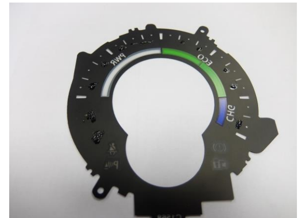
12) Apply small beads of adhesive to the back of the charge/power gauge face taking care to avoid any numbers or markings.
