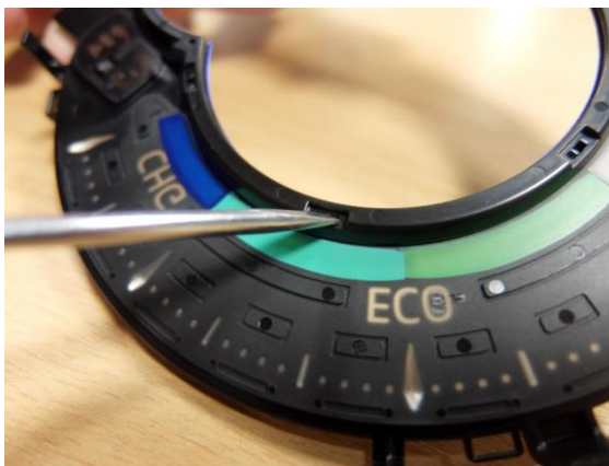
5) Gently press out the clips which hold the blue trim.....
