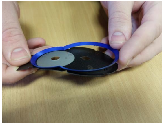
8) Position the blue trim on the new replacement fuel and temperature faces.
