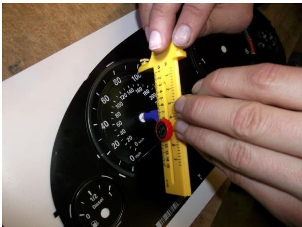
Carefully cut the arc on the pencil mark
