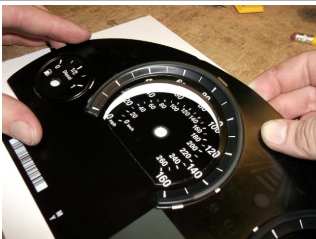
Remove the cut section of dial.....
