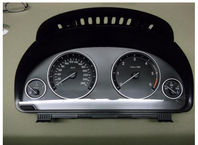
Replace front of cluster and lens
